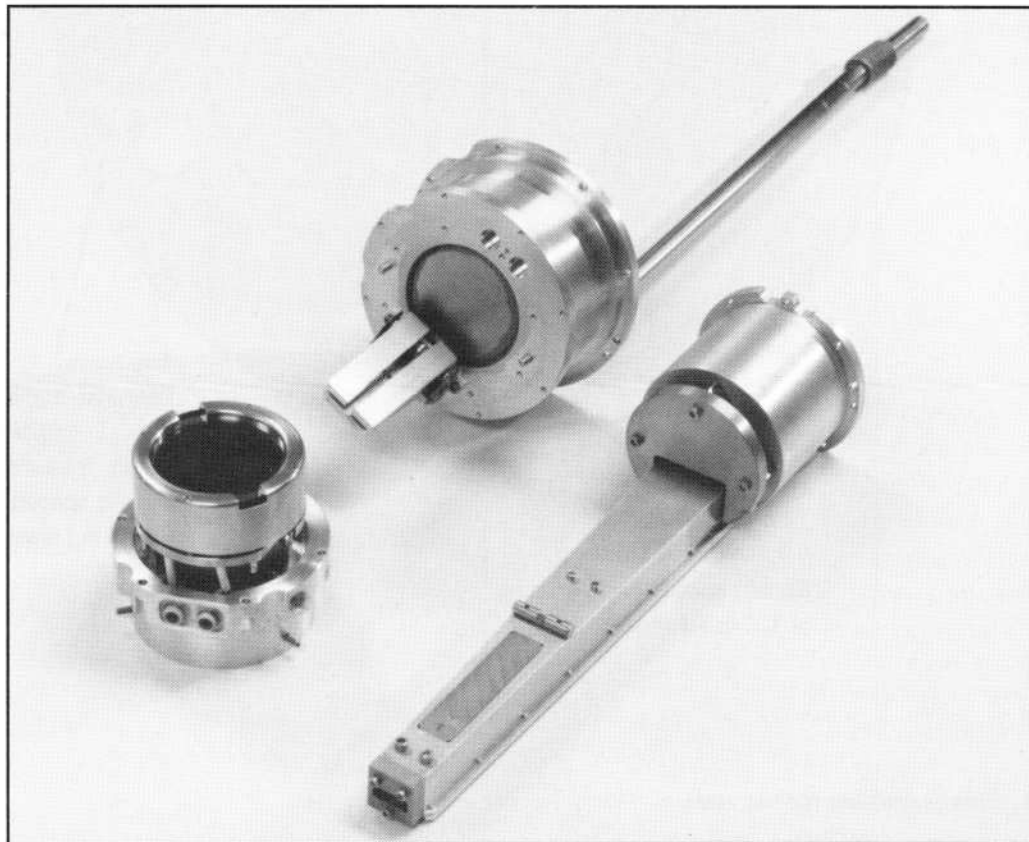
Figure 4. The BrightView imaging subassembly has been used as an imaging element in a special Bragg spectrograph.
